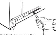
Pull firmly to remove the end of shipping strap from the back of the washer. The shipping strap plug must be completely removed from the washer for the self-leveling legs to be released.
